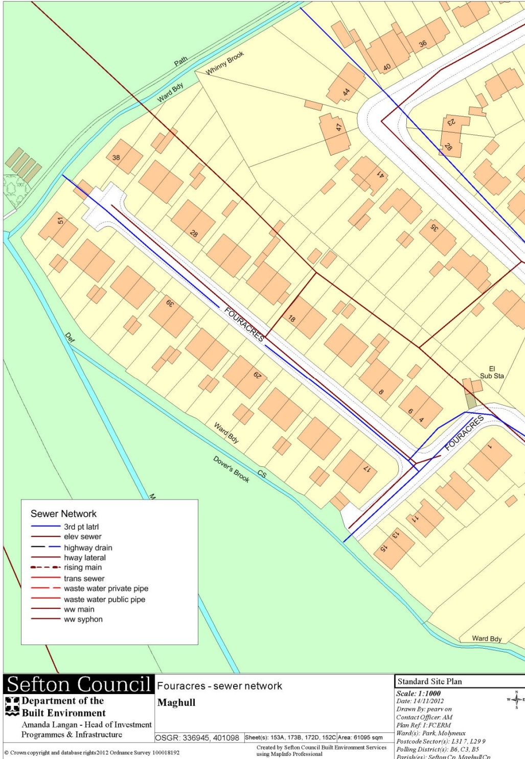
Figure 2: The sewer network
